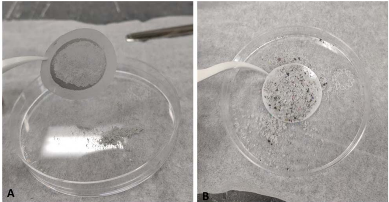
Figure 16. IOM Filters and Bulk Media. A) Bulk Material from Steel Media; B) Bulk Material from Plastic Media
